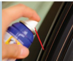
7. Carefully align all components. It is important to operate the window and check for binding before re-installing door panel. Make adjustments where required.
