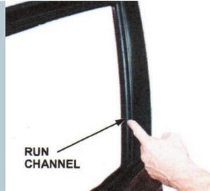
5. Use either a window holding tool or painter's tape to secure the window glass during installation. Do not use strong adhesive tapes like duct tape, as they will leave a sticky residue and can damage the vehicle's paint.
