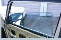
working properly, the windows will lock into position and are held there thanks to the power window regulator assembly. If the window is rolled up but then falls down by itself, this is an indication of a broken regulator assembly. This also tends to happen when the window is crooked, and one side of the window falls down as it's rolled up or down. When this occurs, you'll have to replace the window motor/regulator assembly on most new cars, as they are contained together.
