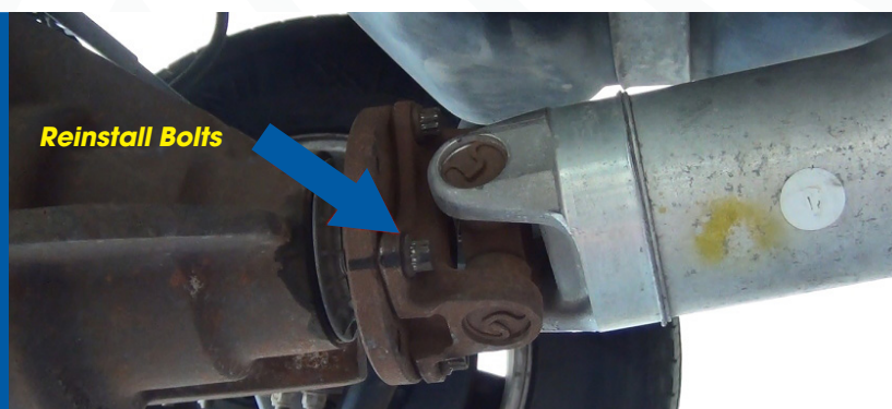
7. Reinstall Flange Bolts
