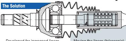
Developed for increased linear travel and greater articulation, to compensate for worn or fatigued engine / transmission mounts.
