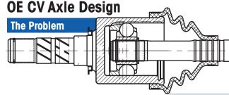
**Developed from Original Equipment** design. These CV axles rely on the inboard joint to provide all linear travel (plunge) for the CV axle.
