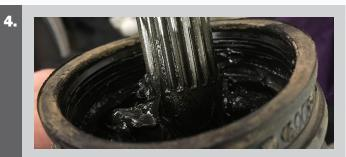
A shudder or vibration when accelerating. This may be caused by play in the inboard or outboard joints, but the most likely cause is a worn inboard joint. Similar vibrations may also be caused by bad motor mounts.
