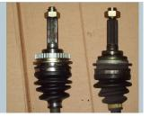
5. Any axle with a circlip on the inner spline should be carefully inspected to ensure no metal pieces / fragments remain in the differential.
