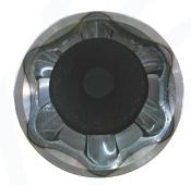
CV joint housings are typically forged from iron billets. After the joint is machined, induction heat treating is used to harden wear surfaces. Wear in a CV joint typically occurs on the cage, gear and cup. This wear is typically caused by a loss of lubrication due to a boot failure, or debris in the joint. Once heat treated surfaces are damaged, they typically cannot be restored.
