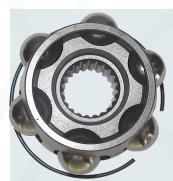
Rzeppa CV joint can be found on the majority of vehicles on the road. A typical Rzeppa joints allow 45°-48° of articulation.
