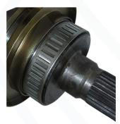
Tone rings are often pressed onto a CV joint. Make sure the number of teeth or windows match the original axle.
