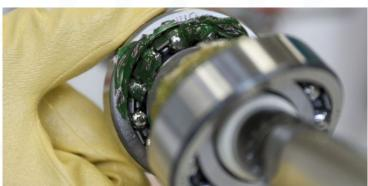
Grease is often packed by hand at the factory. If there is too much grease, the grease will be pushed out of the boot. If you are servicing a joint, use only the recommended amount of grease or only what comes in the kit.
