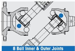
Eliminates joint failure from lift kits and increased ride height. (60% more operating angle on the inboard joint)
