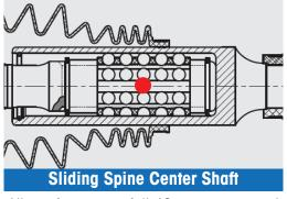
Allows for up to a full 40mm more travel than stock OE units for greater suspension travel for off-road and lifted applications.
