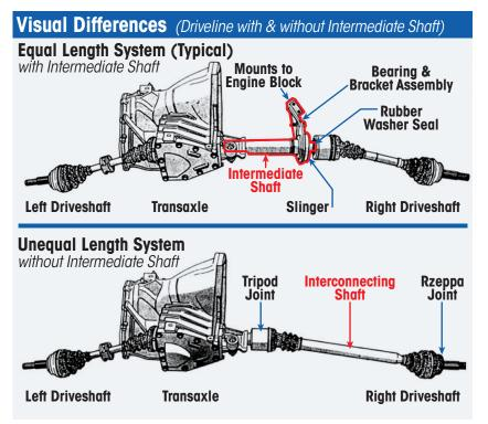
Note: Often, only the intermediate shaft may need to be replaced when the entire CV is initially thought to be at fault. Fix the Cause - Not the Symptom!
